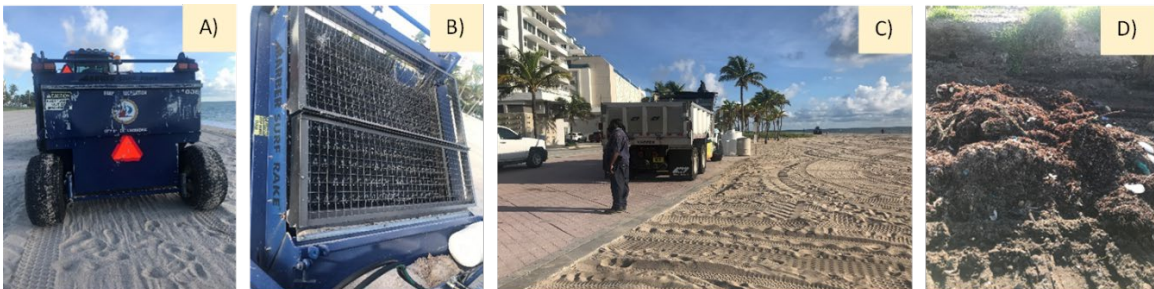
Figure I.1- Barber Surf Rake bucket, where the seaweed is collected. B) Inside of the Barber Surf Rake. C) 8 yd 3 trucks used to empty the Barber Surf Rake. D) Compost pile at Snyder Park.
